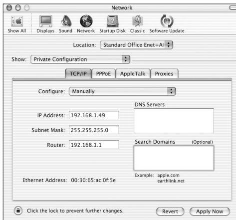
Figure 17.2 Configuring Mac OS X to connect to a gateway for the first time.
